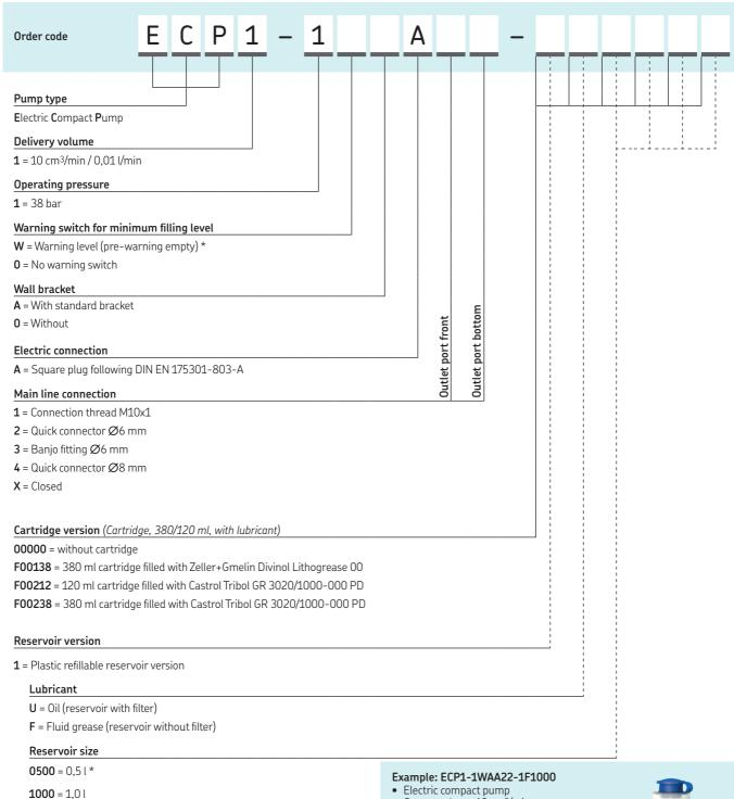
\* NOTE: The 0,5 liter version can not be ordered with warning switch and/or oil filling filter.
